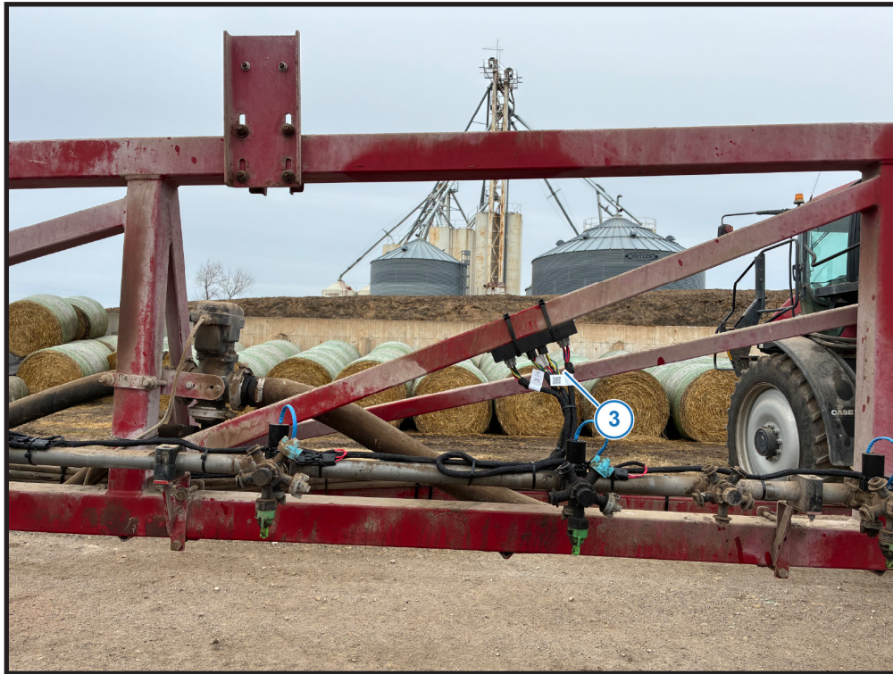
Figure 22: VCM 3 Installation Location
