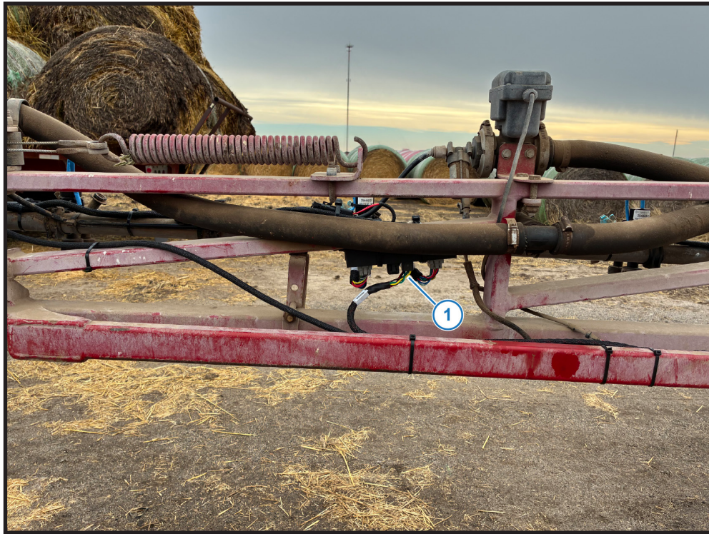
Figure 20: VCM 1 Installation Location
