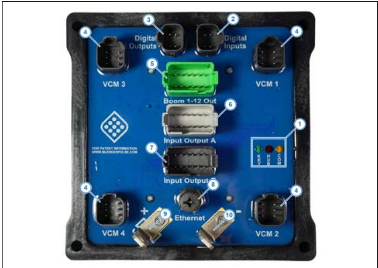
Figure 14: PinPoint III Hub Identification
