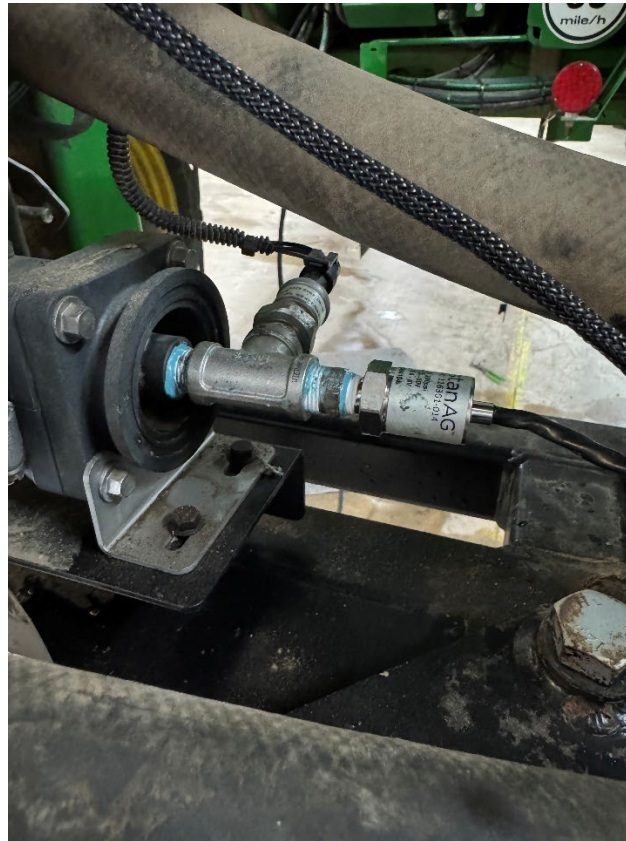
Figure 18. Pressure Sensor Installation (4830 Shown, other models similar)
