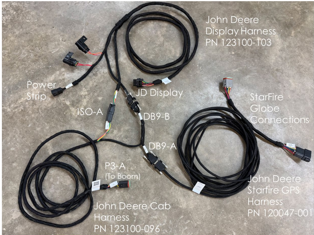
Figure 21. Cab Harnessing and Connections
