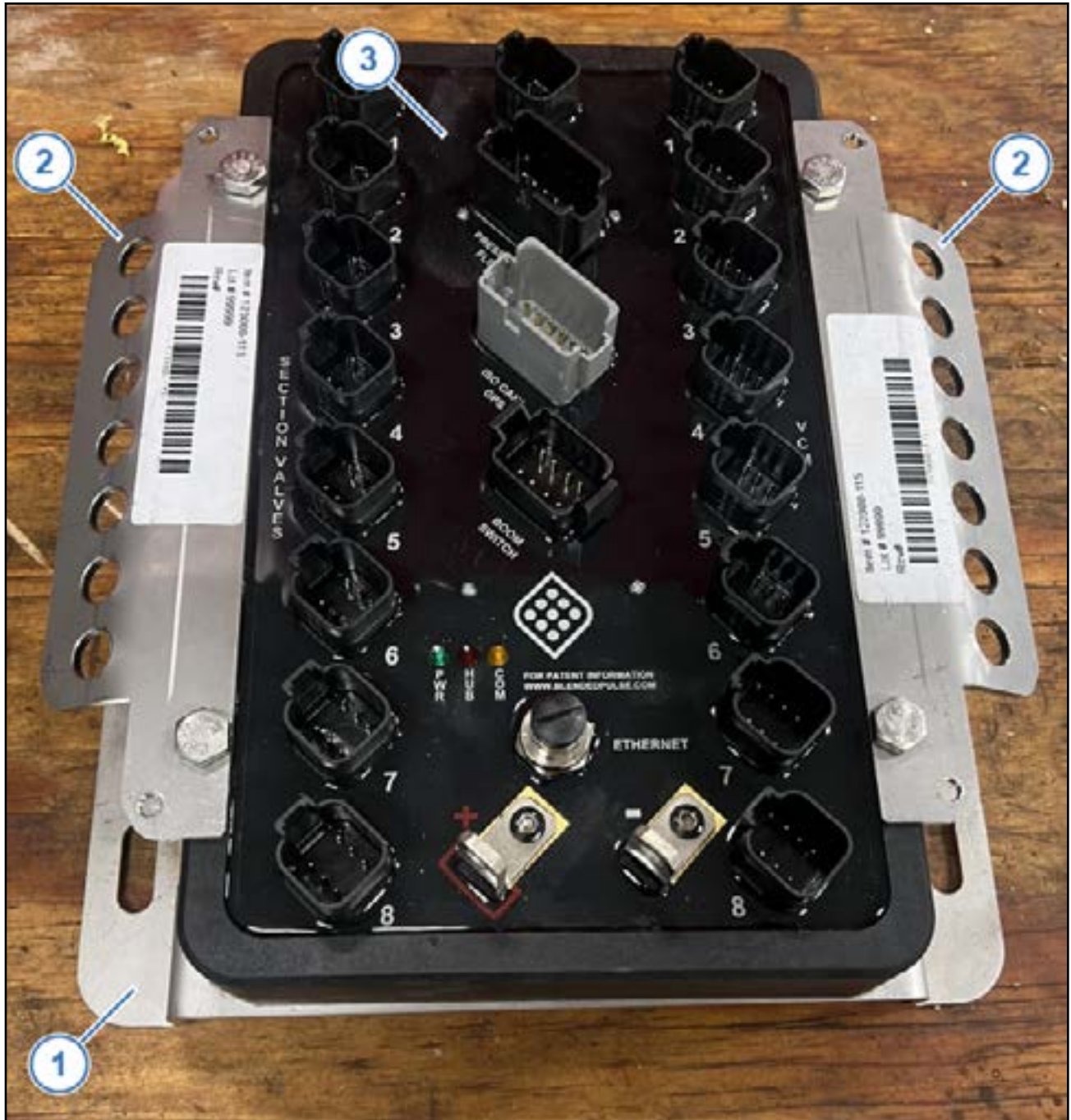
Figure 1: Hub Bracket Installation
