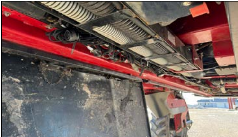
Figure 8: Chassis Harness Routing Example
