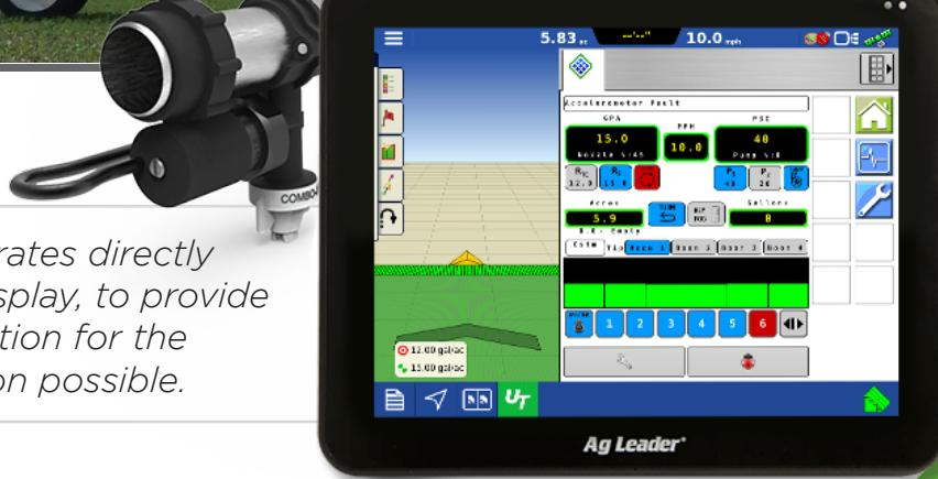
*Pinpoint III ENVELOP integrates directly through the ISOBUS VT/UT display, to provide operator-focused information for the most confident application possible.*
