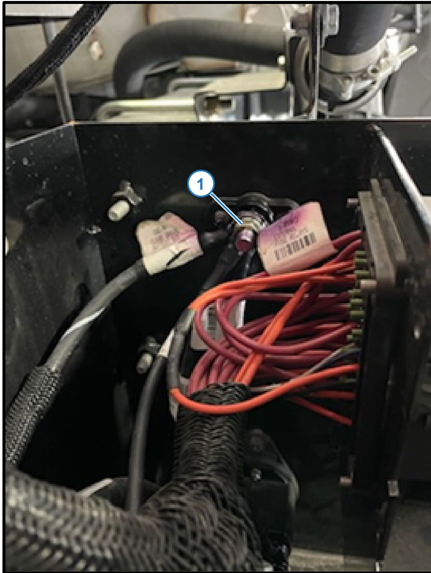
Figure 9 — Negative Power Cable
