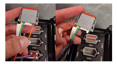
8. Take a 12-pin Deutsch DT male connector and install the orange wire into the pin-6 location and plug all other pin locations.
