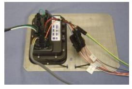
Connect the section harnesses to the valves that are plumbed to the section. Alternate the connections to the valves, white and green across the manifold. Place dust plugs in any unused connectors at the manifold
