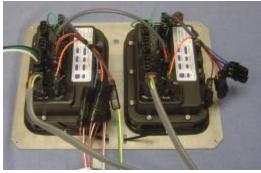
Connect the rate controller harness to the section connections on the Ag Leader/Raven/JD adapter. The servo connection on the second adapter will not be used
