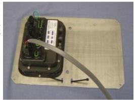
Connect the Ag Leader/Raven/JD adapter to the **SERVO**, **SHUTOFF**, and **CAB POWER** connections on the master module
