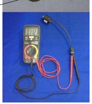
**Single valve will not pulse:** The plunger is lodged with debris or the coil has failed. Check the coil with an ohm meter. The meter should read approximately 12 ohms. Remove coil assembly be careful no to loose the o-ring that seals the coil and the valve body. Check that the poppet is moving freely. Check valve seat for contamination.
