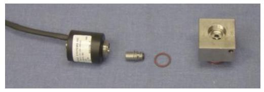
**Single valve will not shut off:** There is contamination in the valve that prevents the poppet from closing completely. Disassemble the valve and remove the contamination. Repeated contamination is a sign of a damaged strainer or improperly sized screen. 80 Mesh is required.
