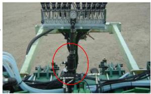
The pulsing valves are ported with a ½" fpt for a hose barb. Using at least 3/8", but preferably ½" hose, connect the valves to the knives or coulters and secure with hose clamps. 1/2" hose barbs are supplied with the manifold. Make sure there is enough slack in the hose for folding and other moving joints. Secure the hoses to the tool bar.
