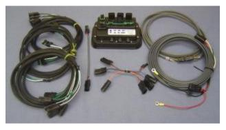
Route the rate controller and power harness across the toolbar so that it will be easy to secure. Remove the hood from the enclosure. The connectors are labeled on the decal. Connect the power harness to the Commander Master Module connector labeled **POWER**.
