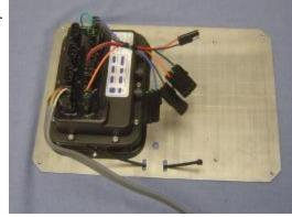
Connect the rate controller harness to the servo and section connections on the Ag Leader/Raven/JD adapter.
