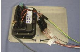
Connect the section harnesses to the **SECTION** connectors on the master module. Route the section harnesses to the manifold.
