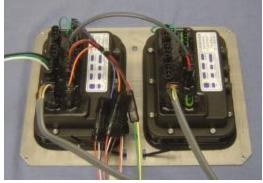
Connect the additional Ag Leader/Raven/ JD adapter to the **SHUTOFF**, and **CAB POWER** connections on the master module. The servo connection on this harness will not be used.
