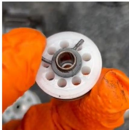
*O-RINGS DAMAGED FROM IMPROPER INSTALLATION
