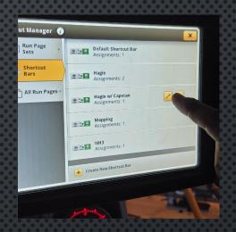
For proper operation of the section control system, a "shortcut" needs to be assigned to enable/disable section control from the run screens. Follow the steps shown here to assign a shortcut
