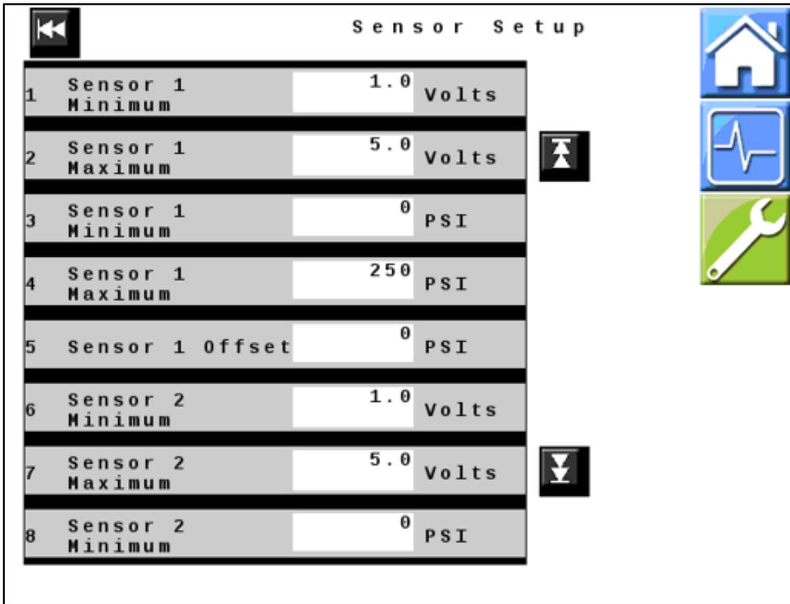
Figure 14 — Sensor Setup Page 1 (OEM Pressure Sensor)
