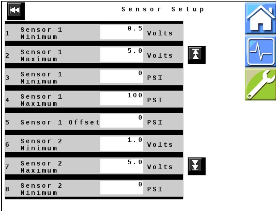
Figure 13 — Sensor Setup Page 1 (Capstan Pressure Sensor)
