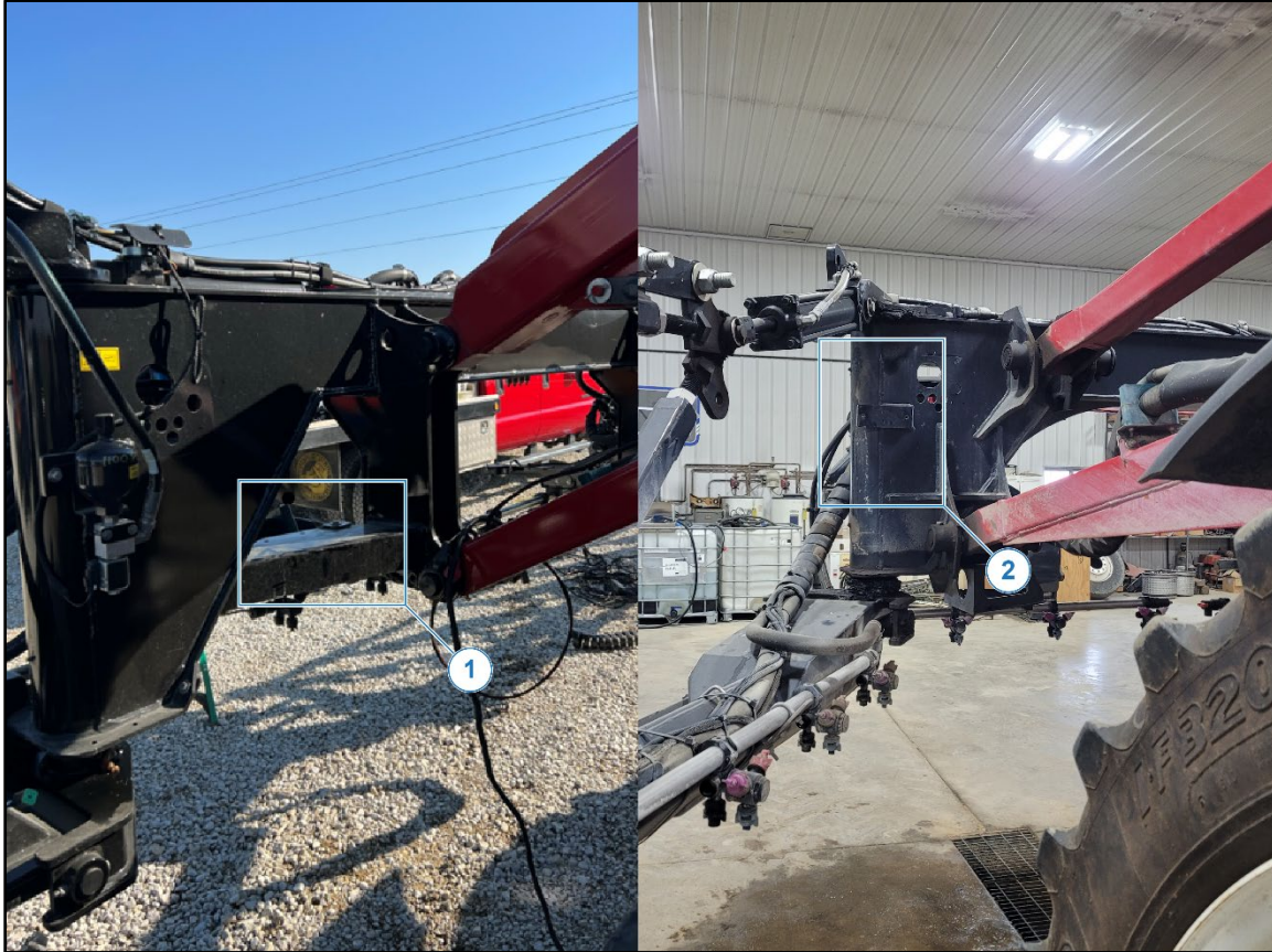
Figure 1 — Envelop Hub Mounting Location
