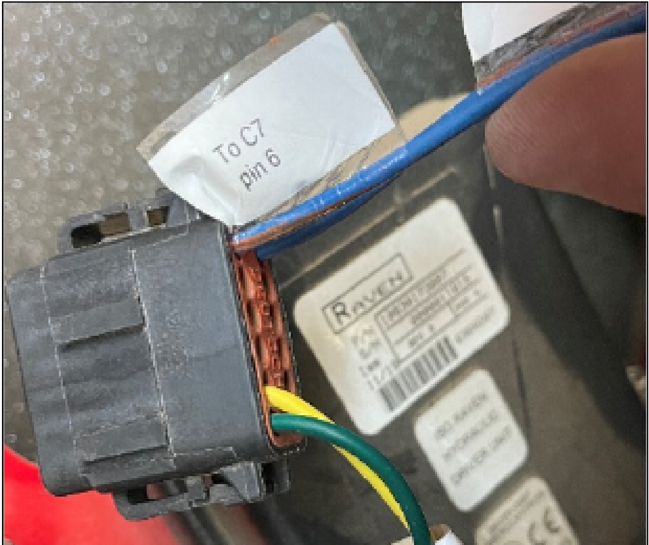
Figure 8: C7 Plug Detail
